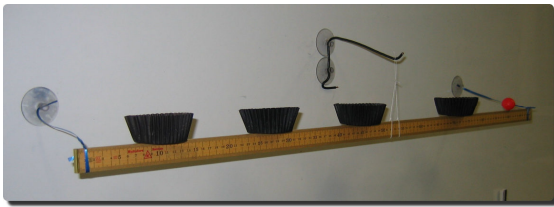
Figure 2: Setup to drop stacked paper cups simultaneously.
